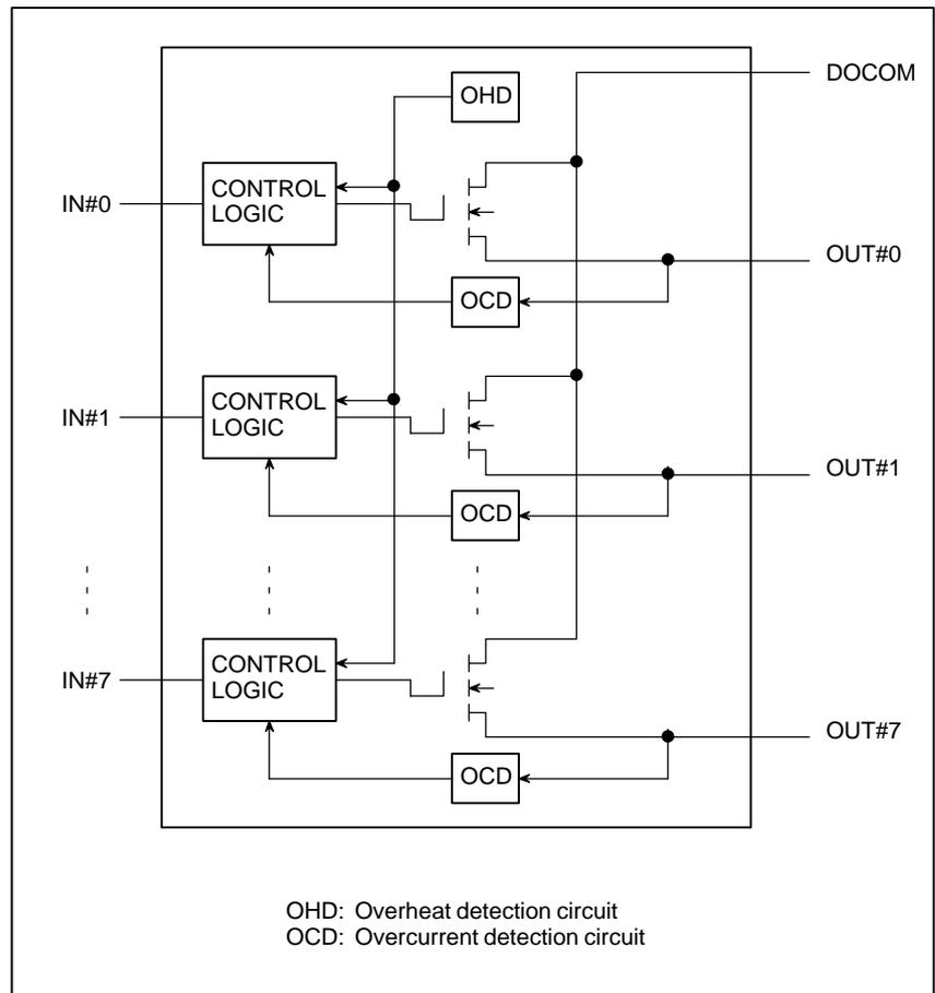
The power for operating this driver element is supplied from DOCOM (24 VDC).
