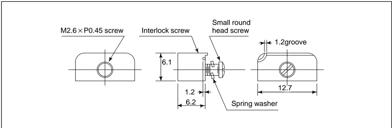
Fig. C8 (b) Locking plate for reader/puncher interface connector
