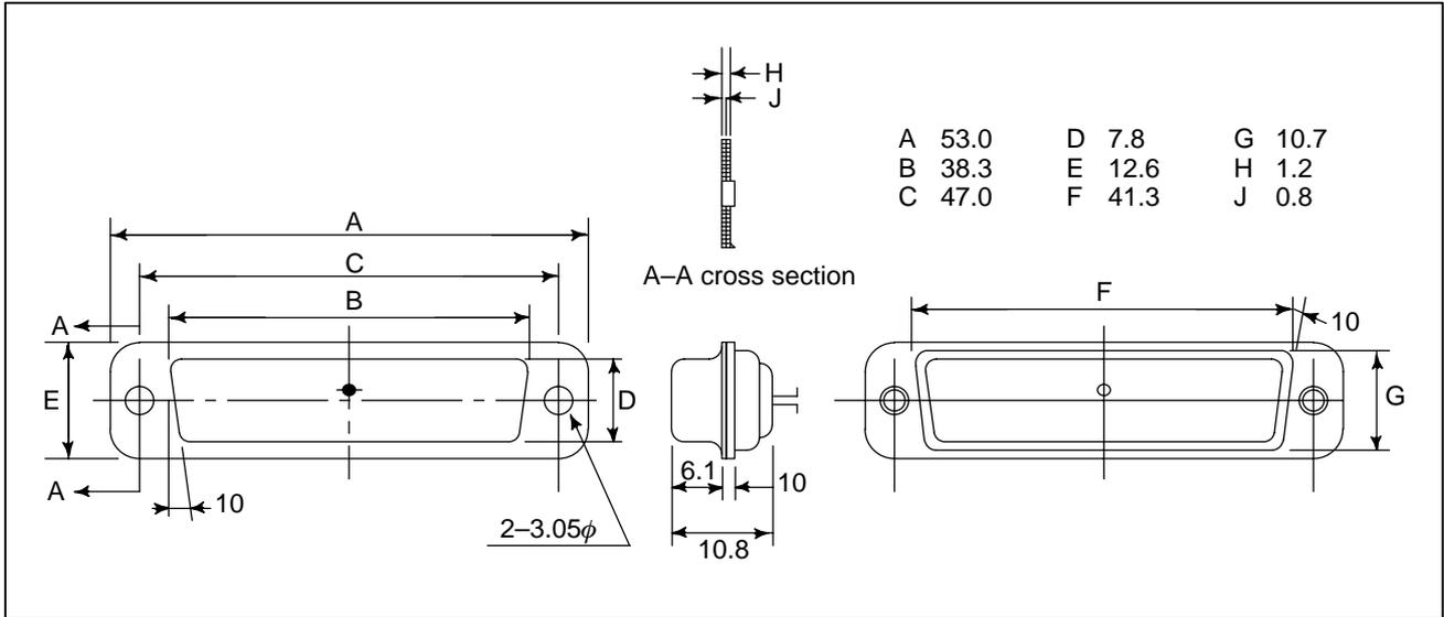
Fig. C8 (a) Punch panel connector for reader/puncher interface
