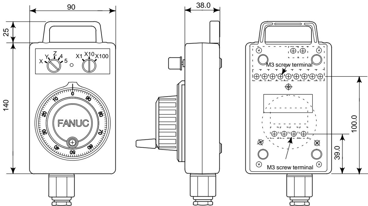
Fig.U19 Pendant type manual pulse generator
