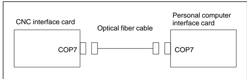
Compatible cables (optical fiber cables, used for interconnections)
