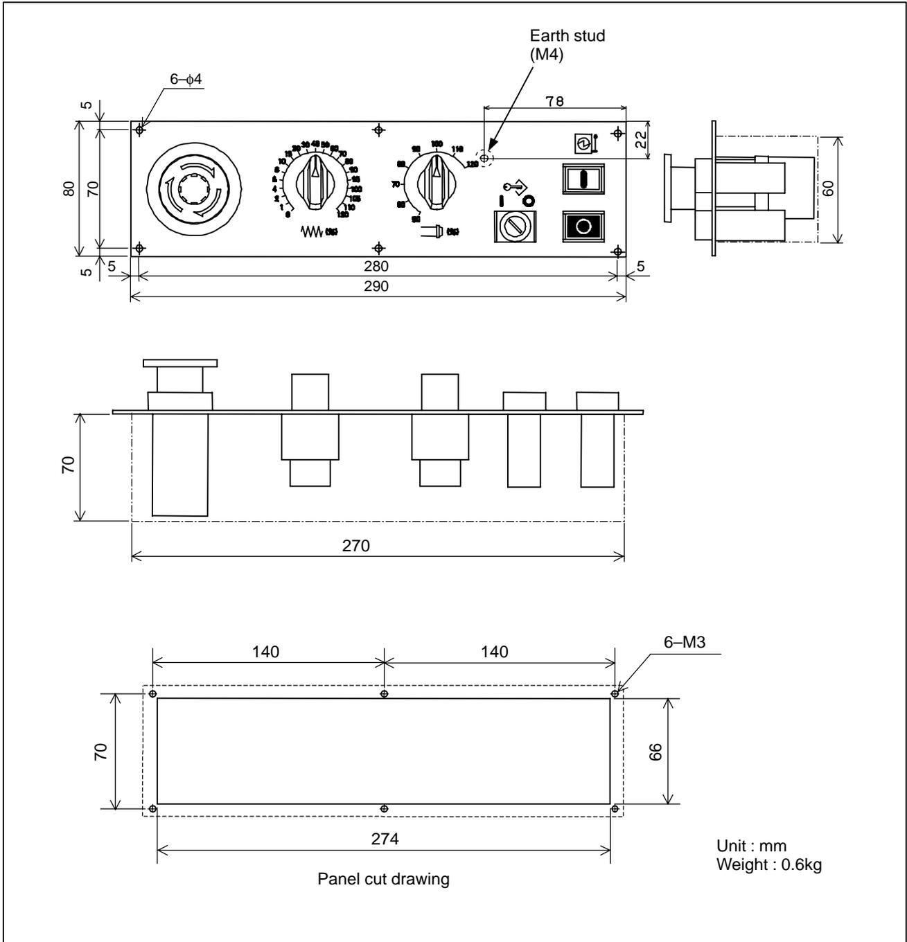
**Fig.U26 Machine operator's panel (Sub panel A)**
