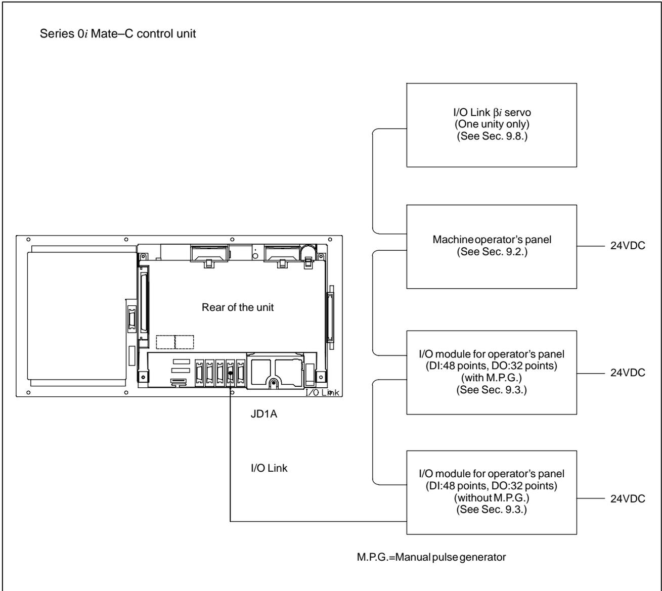
The following is an example in which two operator's panel I/O boards and one machine operator's panel are used.
