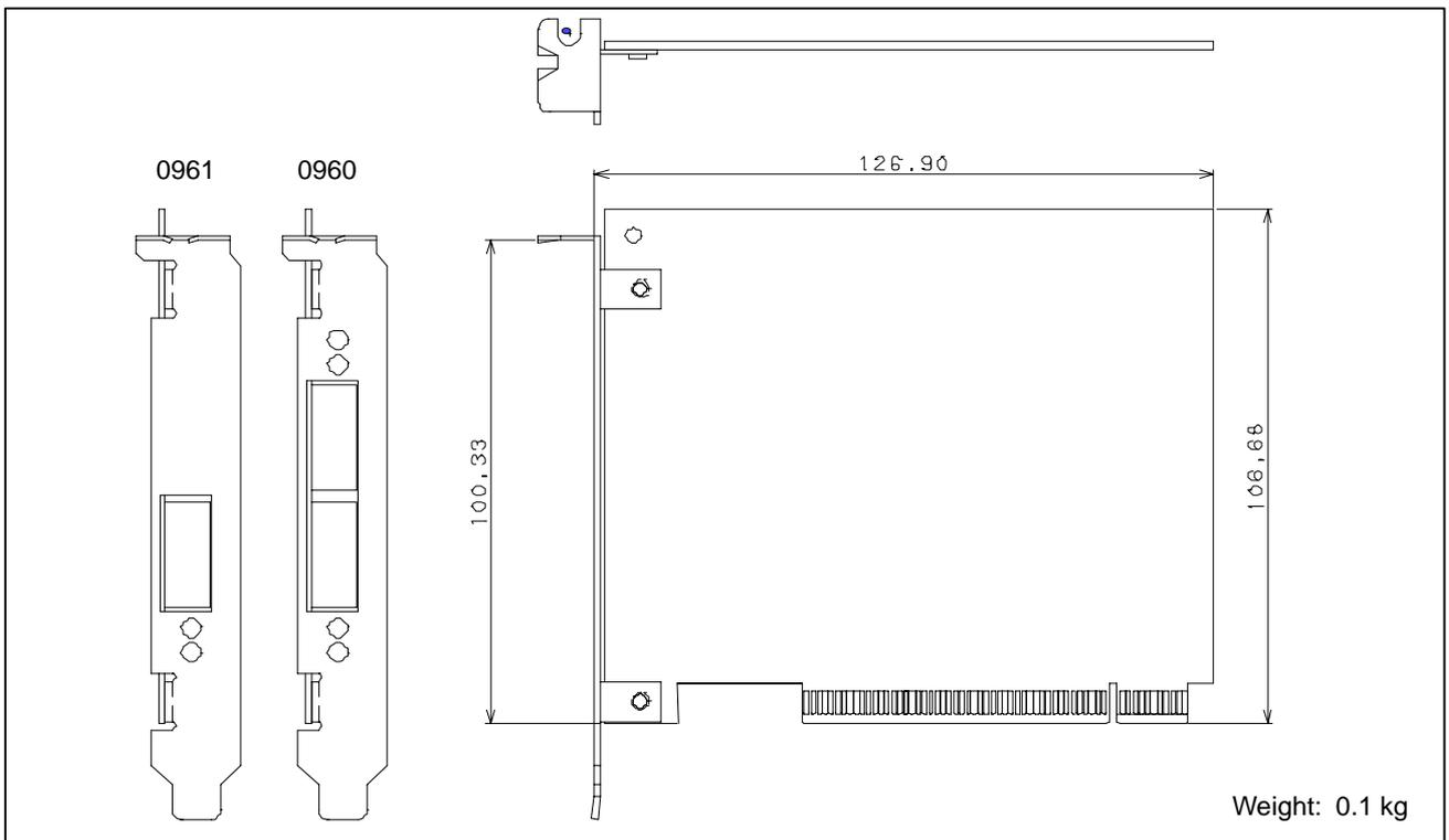
**Fig.U16 (b) Interface Board for Personal Computer (PCI bus version)**
