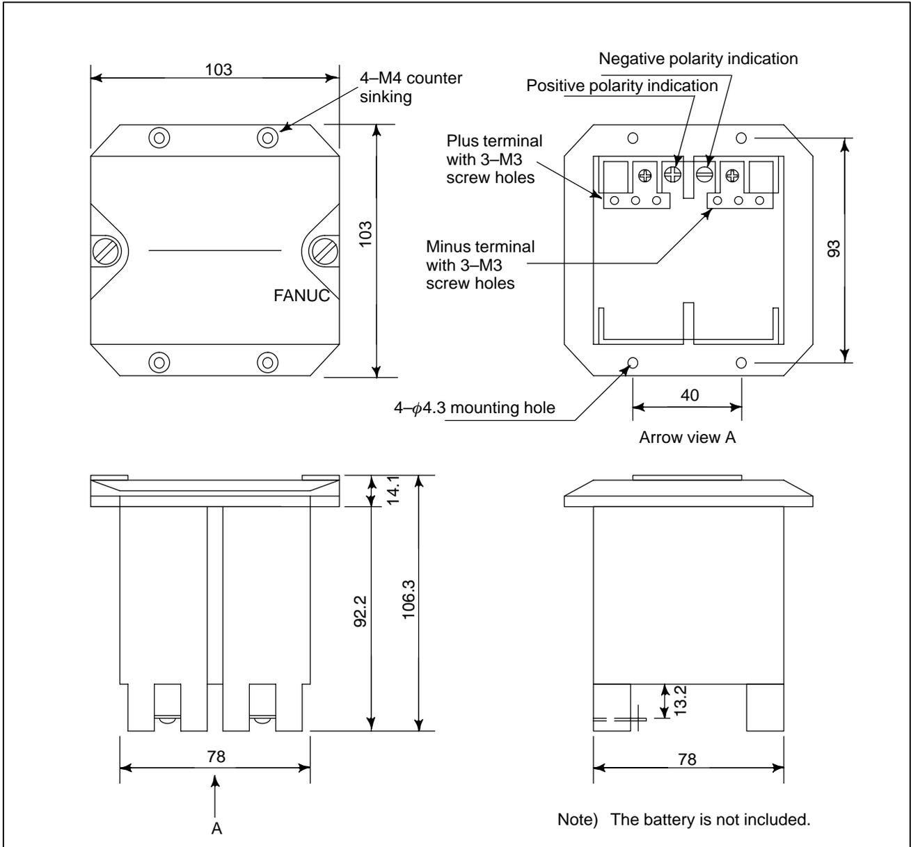
**Fig.U21 External dimensions of ABS battery case for separate detector**
