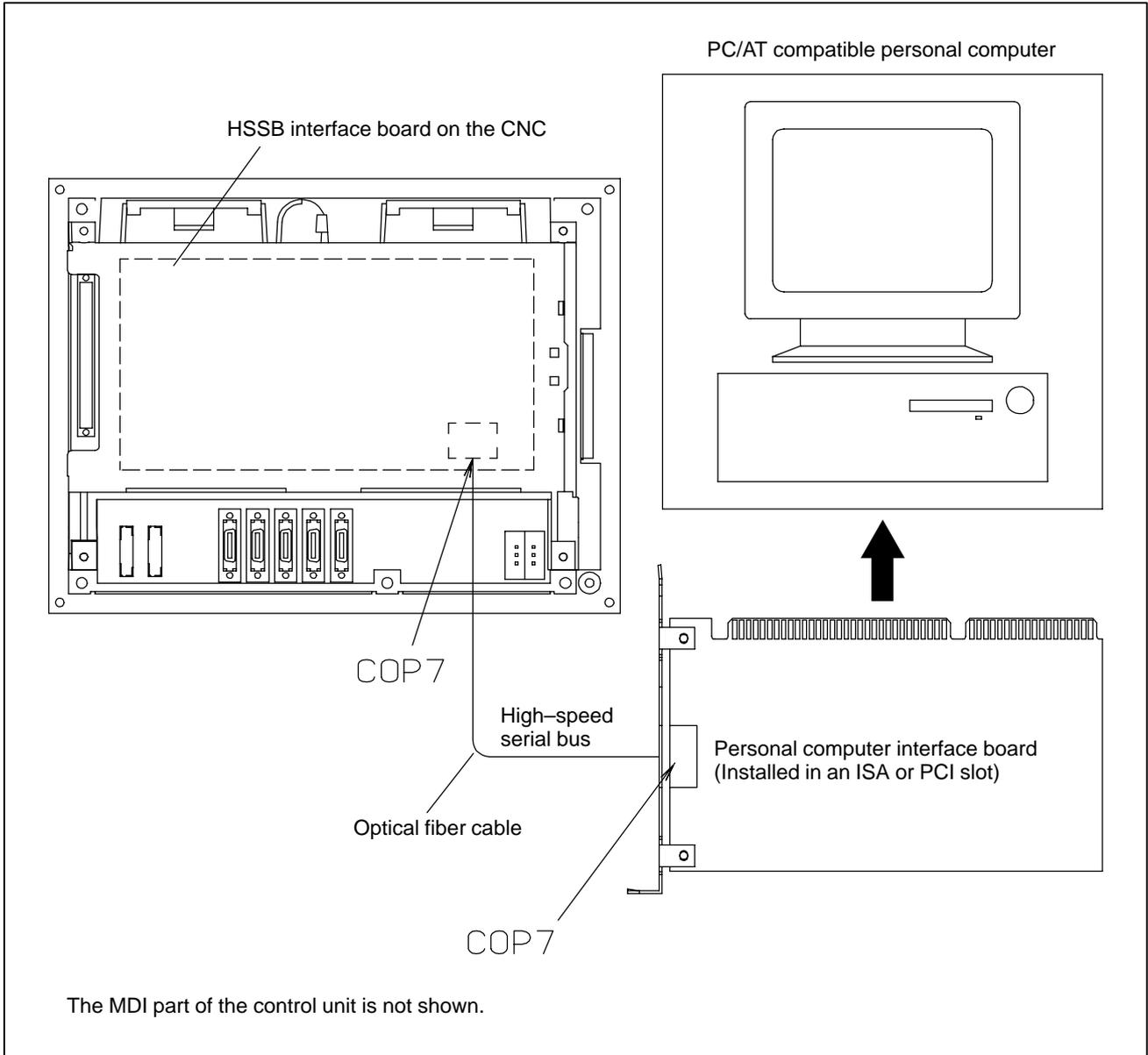
The PC interface boards include an ISA bus interface board and a PCI bus interface board.
