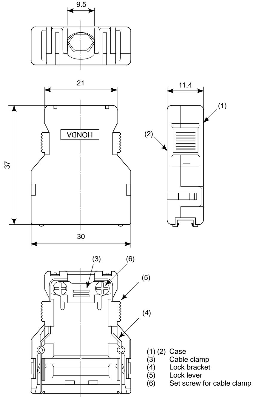
Fig. C2 (a) Connector case (HONDA PCR type)
