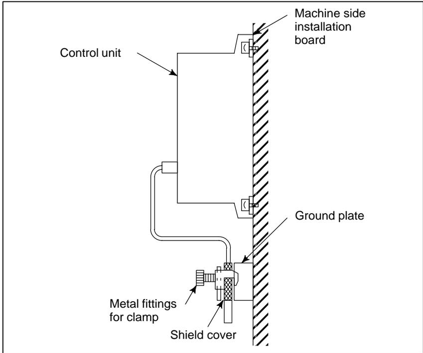
**Fig. 3.5.5 (b) Cable clamp (2)**
