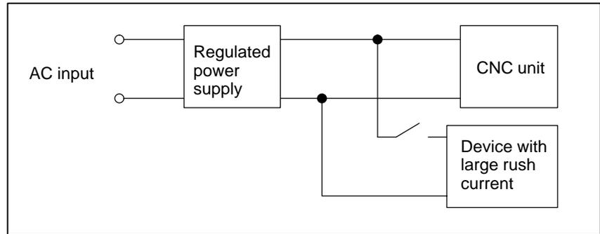
For a circuit configuration in example 2, connect another regulated power supply to be specifically used for the device with remarkable load fluctuations so that the CNC and other units are not affected.
