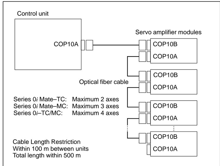
The connection between the CNC control unit and the servo amplifiers should use only one optical fiber cable, regardless of the number of controlled axes. See APPENDIX D for details on the optical fiber cable.
