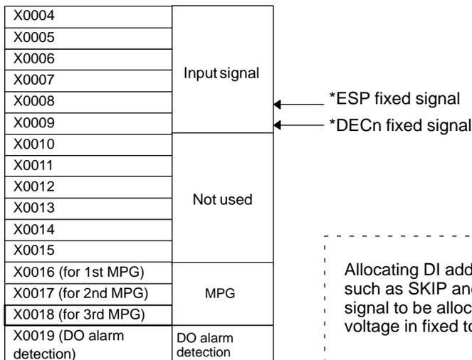
Allocating DI addresses from X0004 allows the fixed signals, such as SKIP and \*DECn, to be used and the \*ESP fixed signal to be allocated to an address for which the common voltage is fixed to 24 V.
