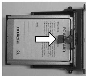
Insert the memory card into the fixing bracket in the direction indicated by the arrow.
