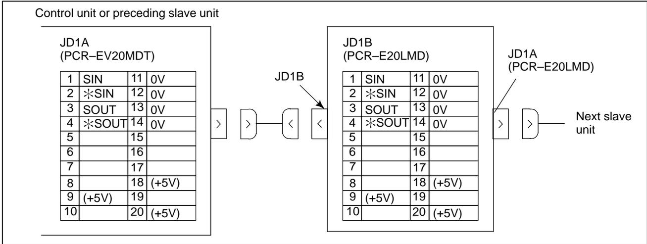
+5 V terminals are for an optical I/O Link adapter. They are not necessary when connecting with a metal cable.
