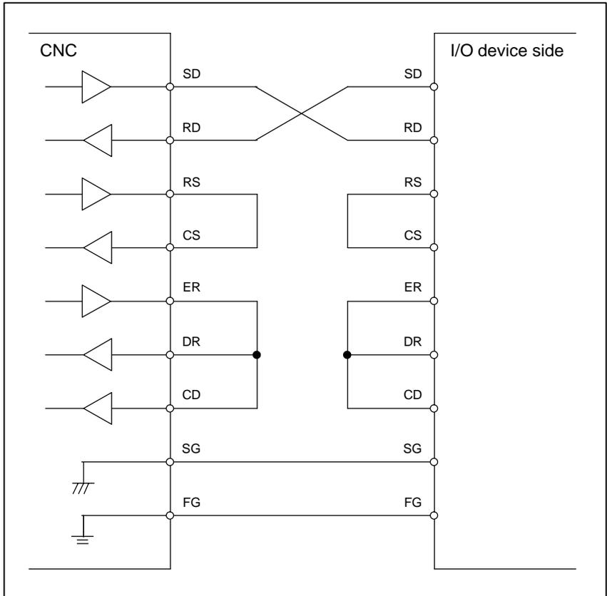
Prepare the cable with I/O device as follows :
