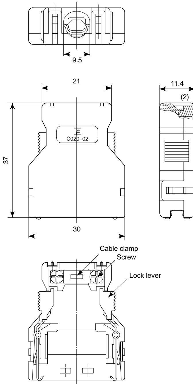
Fig. C2 (c) Connector case (FUJITSU FCN type)
