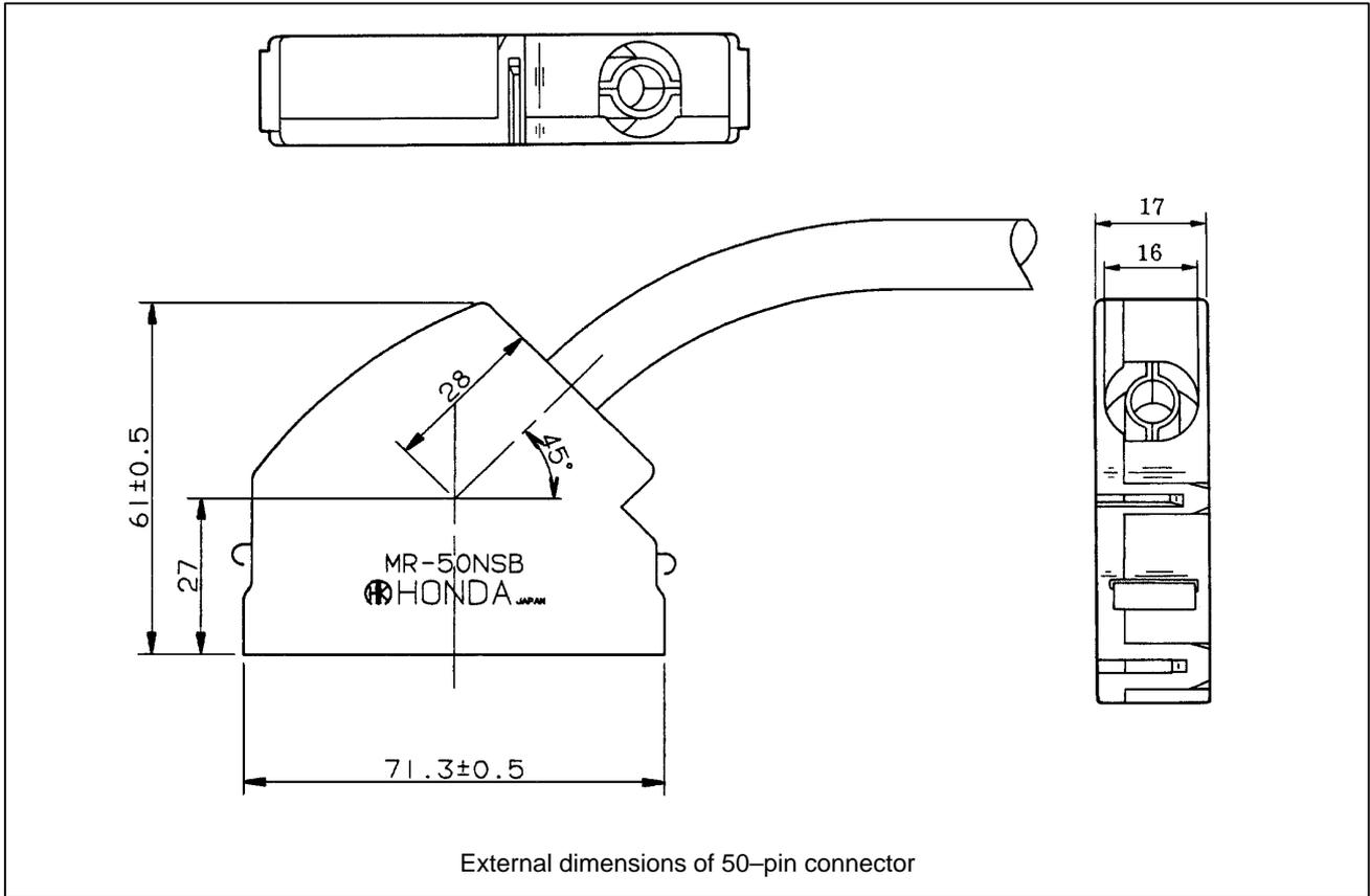
**Fig. C4 (b) Honda connector (angled-type case)**
