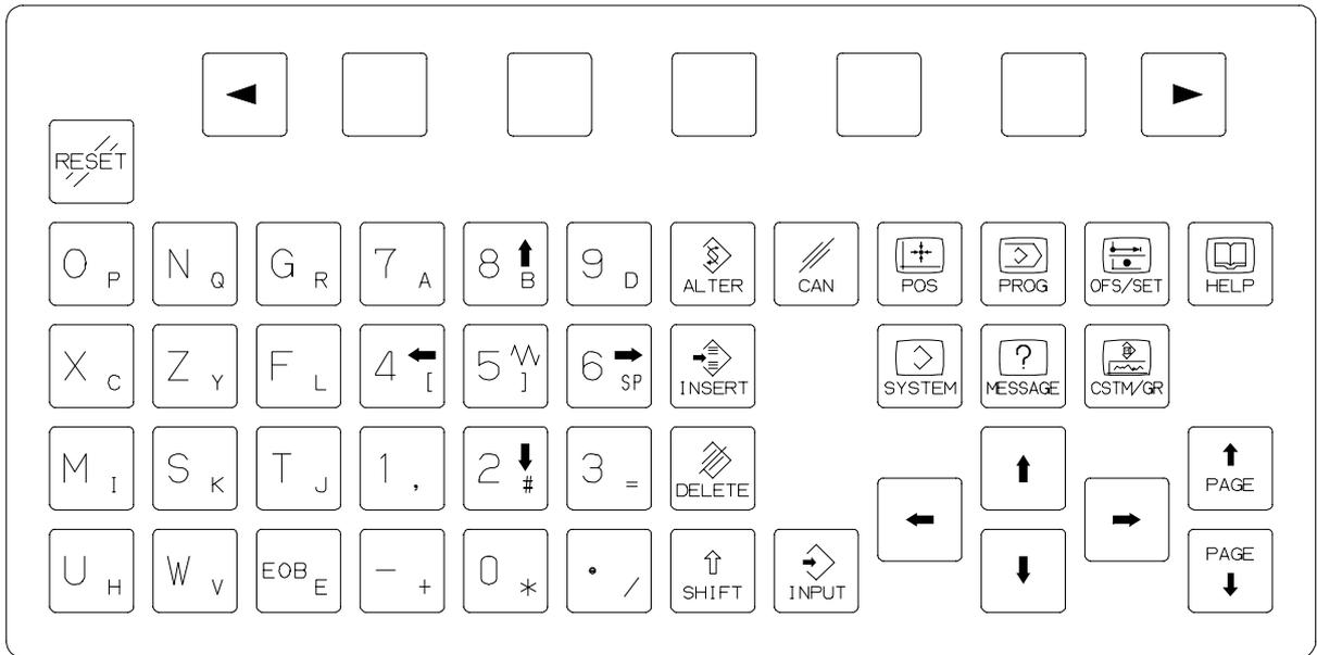
**Standard keys for machine center series (M series) (vertical type)**
