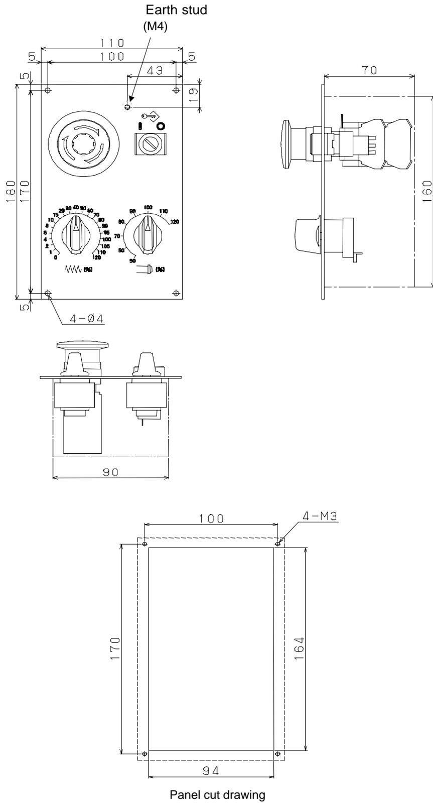
Fig.U27 Machine operator's panel (Sub panel B1)
