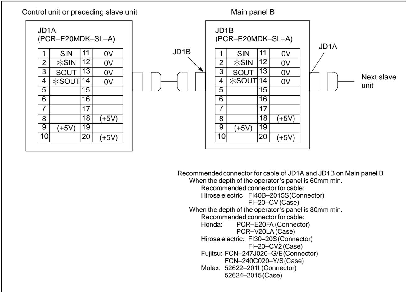
+5V terminals are for an optical I/O Link adapter. They are not necessary when connecting with a metal cable.
