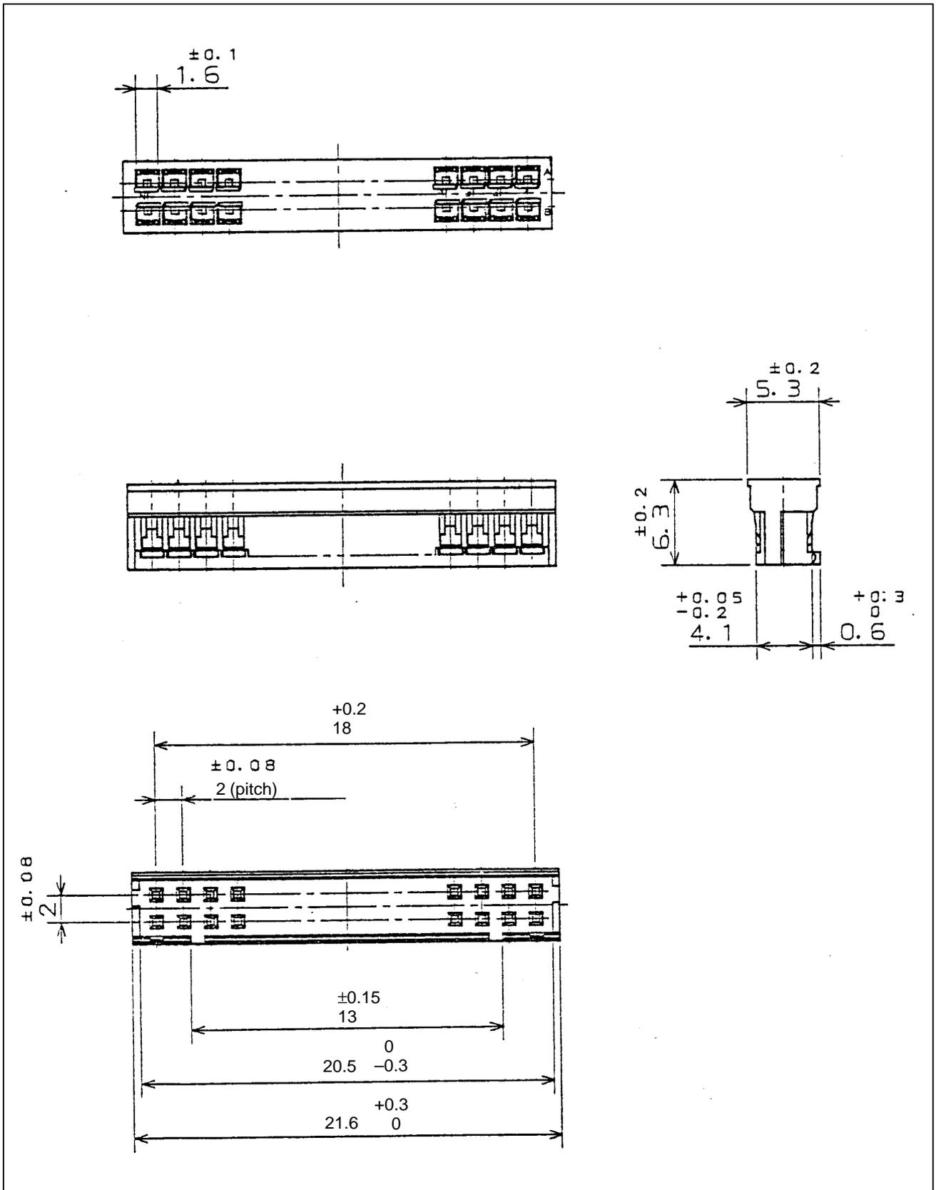
Fig. C7 (a) Connector (Japan Aviation Electronics)(for MDI)
