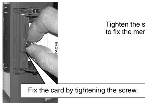
Tighten the screw of the bracket to fix the memory card.
