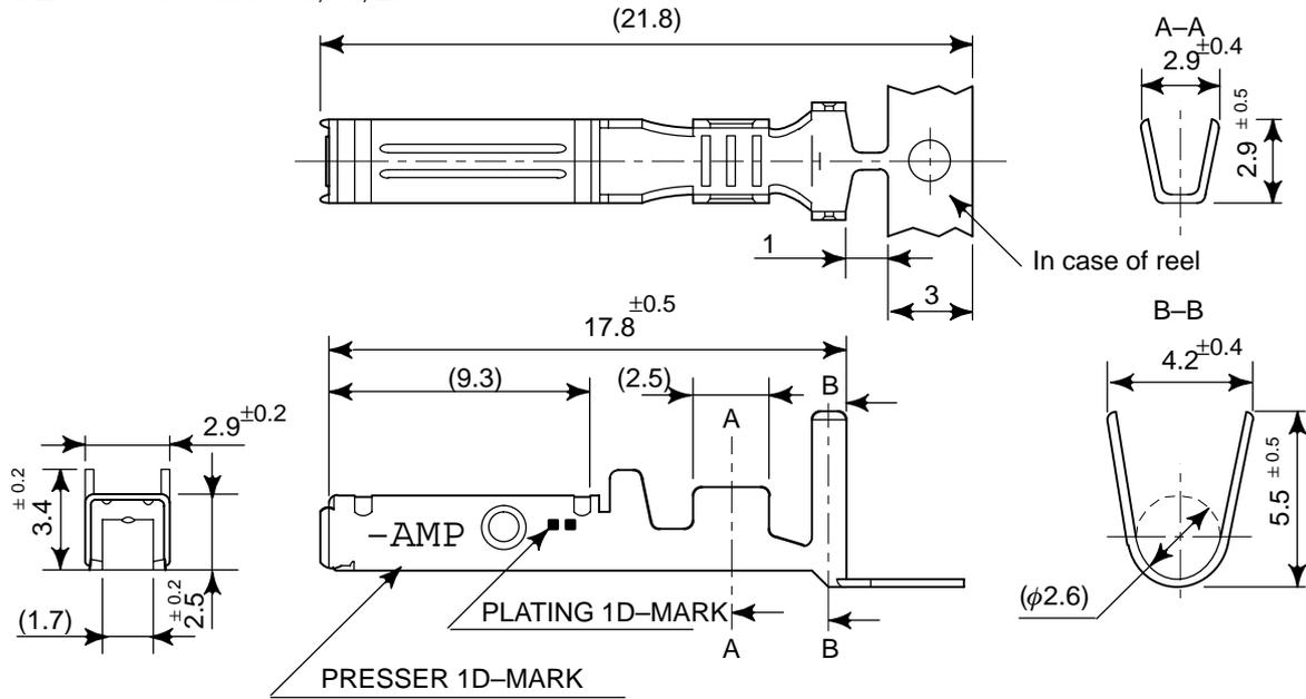
Fig. C3 (e) Contact for AMP connector
