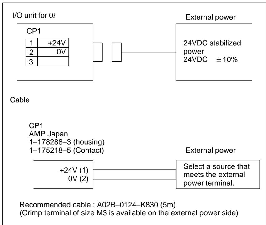
Part of the 24 VDC power input to CP1 can be taken out from CP2 by branching. CP2 should be connected as shown below. In this case, the rating of the external 24 VDC power supplied to CP1 must be the sum of the power consumed within the control unit and that supplied to external equipment via CP2. The maximum capacity of power that can be obtained from a branch is 1.0 A.
