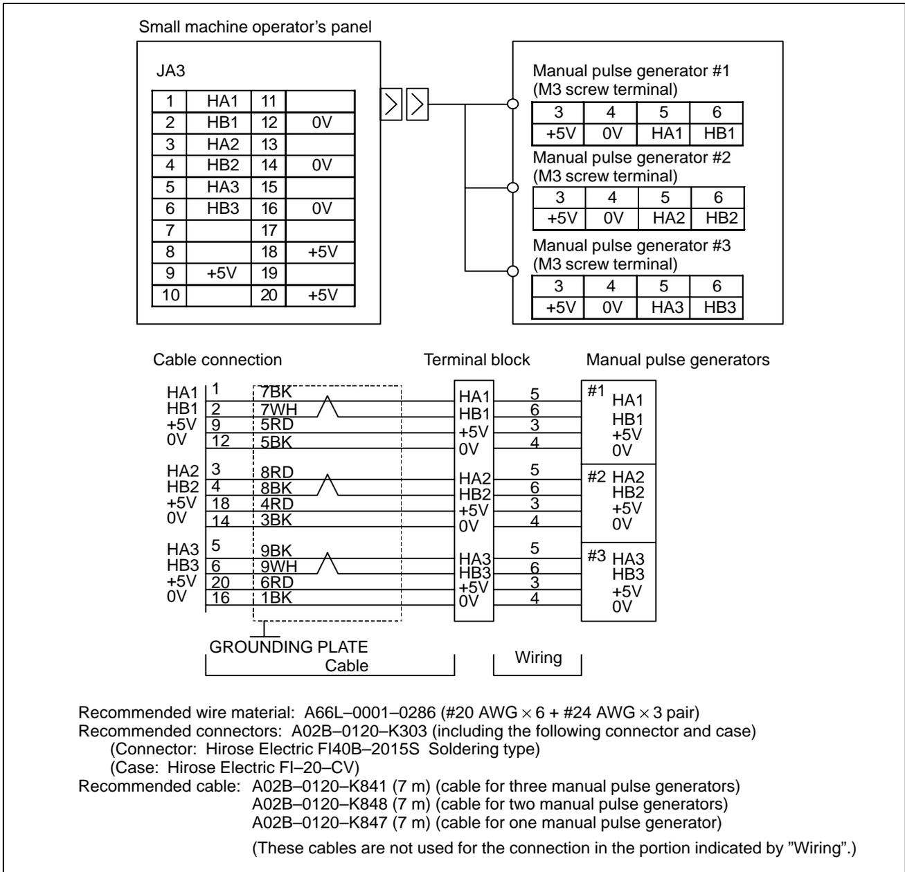
Calculate the maximum allowable length of the cable for the manual pulse generator, with the method described below.
