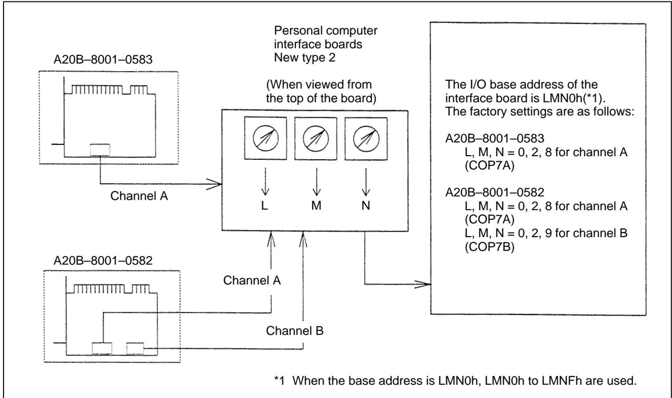
Fig. 11.6 I/O base address setting (for personal computer interface board of new type 2 (A20-B-8100-0582, -0583))
