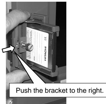
Align the claw of the fixing bracket with the groove of the PCMCIA port and then push the bracket in the direction indicated by the arrow.
