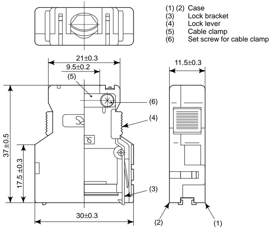
Fig. C2 (b) Connector case (HIROSE FI type)
