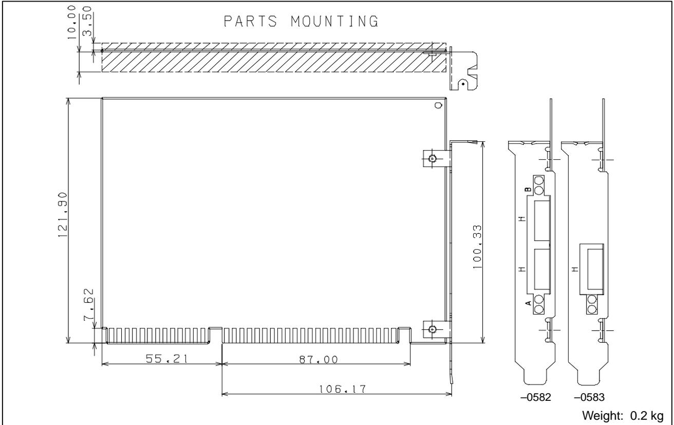
**Fig.U16 (a) High-speed serial bus interface board type 2 (PC) (ISA bus version)**
