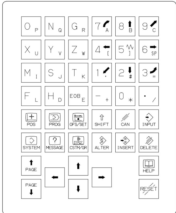
**Standard keys for lathe series (T series) (vertical type)**
