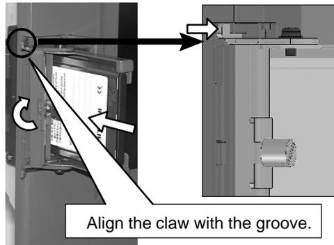
Loosen the screw of the fixing bracket and insert the memory card into the PCMCIA port with the claw of the fixing bracket raised.
