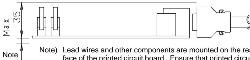
Note) Lead wires and other components are mounted on the rear face of the printed circuit board. Ensure that printed circuit boards are spaced 5 mm or more from one another to prevent interference.
