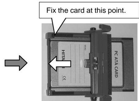
Fix the memory card to the fixing bracket.
