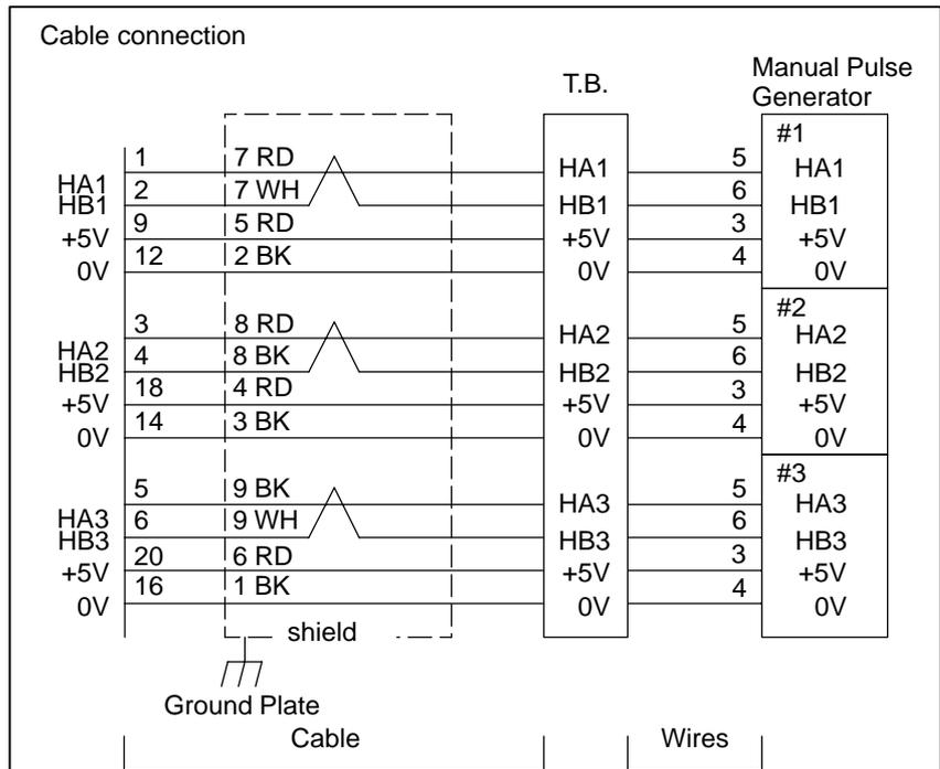
Recommended Cable Material (See Appendix B for details of cable material.)
