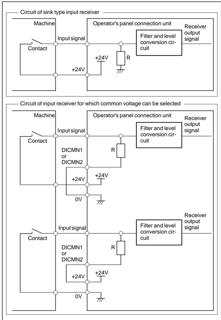
Fig. 9.7.1 (a) Receiver circuit
