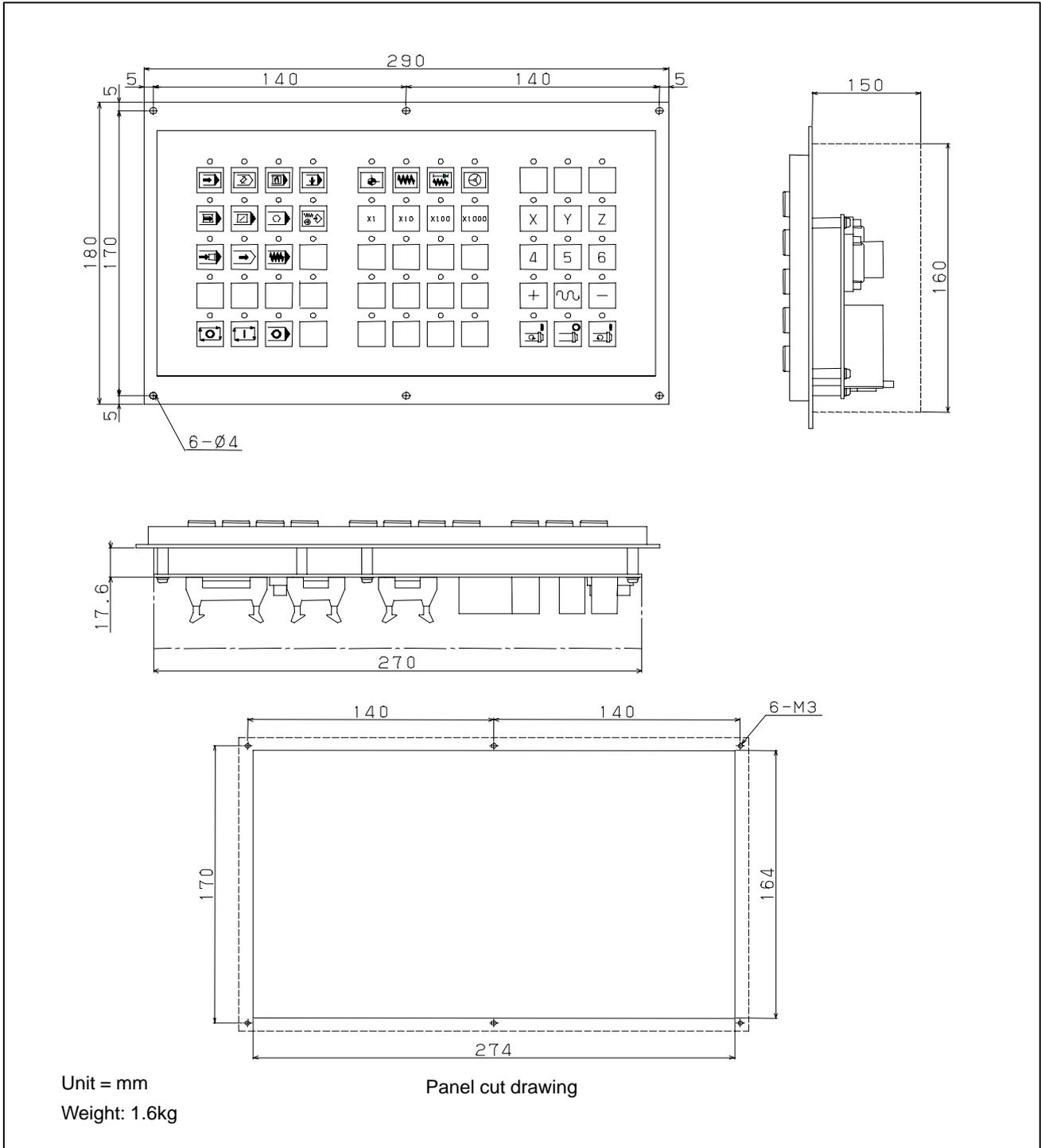
**Fig.U25 Machine operator's panel (Main panel B)**
