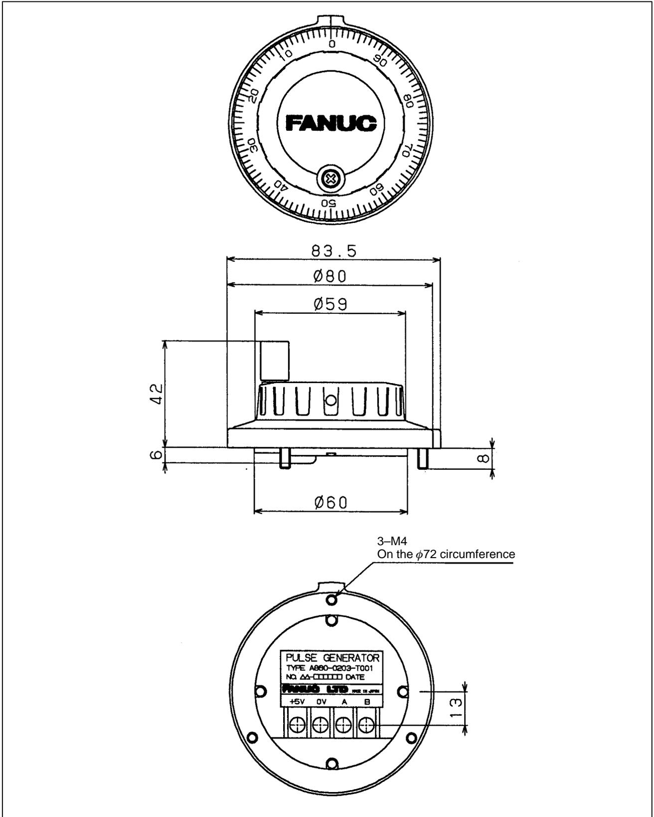
Fig. U24 External dimensions of manual pulse generator
