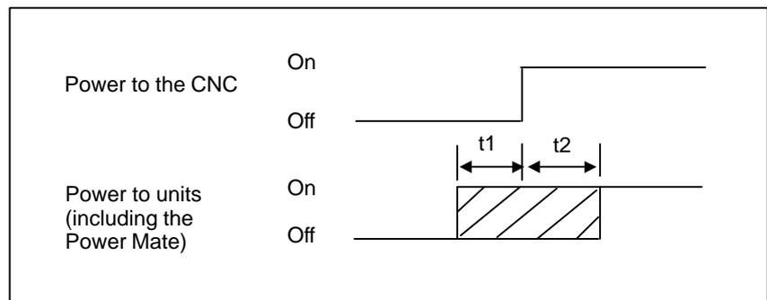
$t_1 : 200 \text{ ms}$  Means that the power to units (including the Power Mate) is turned on within 200 ms before the power to the CNC is turned on.
